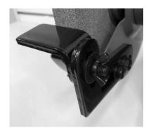
Attach the tool rest (A) to the bracket (B) using the long fastener (G) and the Large Washer (C) and wing nut (D). then attach this to the bench grinder using the 2 x small washers (E) and 2 x short fasteners (F), allowing no more than 2mm gap between the grinding wheel and tool rest (A).
