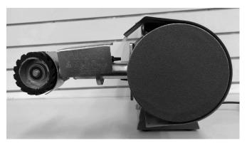
Attach the abrasive disc (C) to the backing plate. Hold firmly for a few seconds to ensure the adhesive activates.
