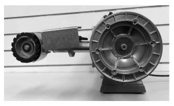
Place the Drive Pulley (H) onto the shaft of the bench grinder if it is a 16mm dia shaft. If the bench grinder has a smaller 12mm shaft you will need to insert the bush (not pictured) to the shaft and then place the drive pully onto the shaft to ensure there is a snug fit.
