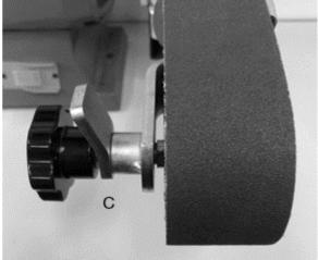
Turn the unit on and inspect the movement of the belt. If adjustments are required move the lever into the loose position (A) To correct any tracking concerns simply turn the knob (B) to adjust the tracking and once adjusted lock the lever gently back into place (C).
