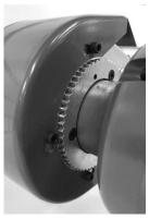
Attach the abrasive disc (C) to the backing plate. Hold firmly for a few seconds to ensure the adhesive activates.
