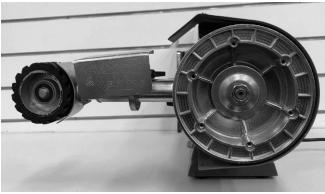
Install the guard (F) over the assembly and tighten the 3 x 6mm cap screws (G)
