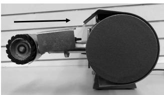
Push against the contact wheel towards the drive pulley to retract the extension arm and place the linishing belt (B) over the main wheel and the contact wheel. Refer to the inside of the belt for the correct installation direction of the belt.
