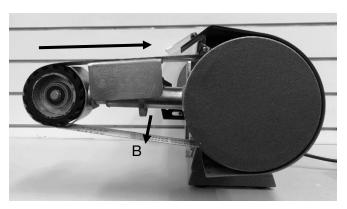
Push against the contact wheel again to extend the extension arm. Ensure the belt is taught and not loose.
