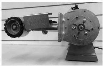
Install the Main Bracket (A) to the Grinder, using the 3 x 6x20mm locking fasteners (I)
