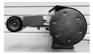
Install the backing plate (D) to the drive pulley with the 6 x fasteners (E)
