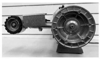
Place the washer (K) over the shaft onto the drive pulley
