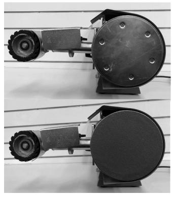
Install the guard (F) over the assembly and tighten the 3 x cap screw (G)
