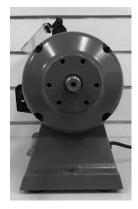
Remove the grinding wheel and guard off the side of the bench grinder that you would like to install the linishing attachment to. Keep the original nut and washer holding the grinding wheel in place
