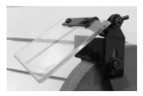
Use the wing nut (D) and 1 x washer (B) secure the eyeshield to the bench grinder allowing no more than 2mm gap between the grinding wheel and bracket (A)
